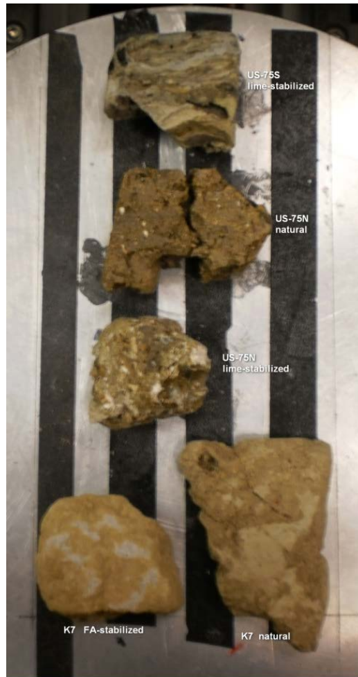
Figure 13. Prepared SEM samples from test sites in Kansas
