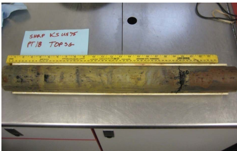
Figure 12. Shelby tube sample after extraction
