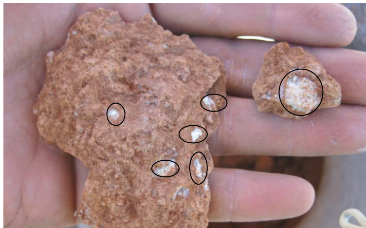
Figure 14. White product presented in stabilized subgrade at test site of US 183
